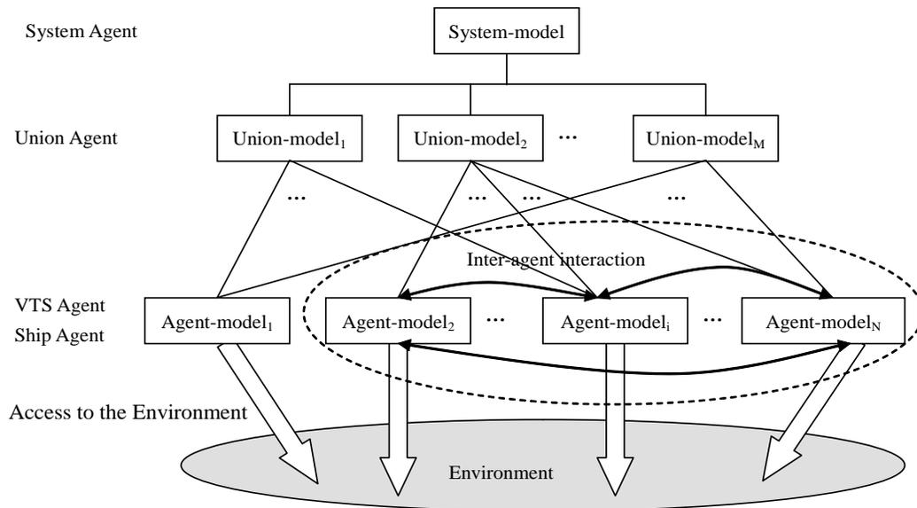
**Figure 1: The architecture of multi-agent system for collision avoidance**
