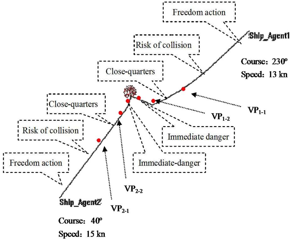
Figure 3: A dynamic course of a collision case
